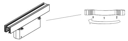
2. Then turn the LOCK handle counterclockwise to switch from "LOCK" to "UNLOCK".
