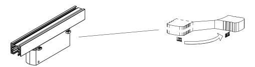
3. Finally, pull down one end of the guide light connector to remove the entire guide light connector.
