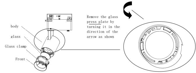
b. Put the new glass into the lamp, and put the glass pressure plate into the lamp, and press tightly according to the following figure;;
